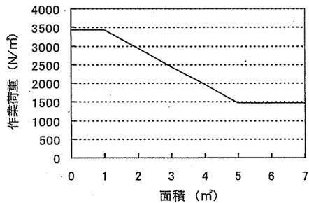
Fig. 17 The surface areas and specified working loads.
