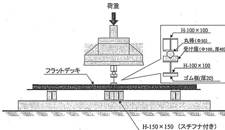
Fig.11 Supporting test for ribs.
