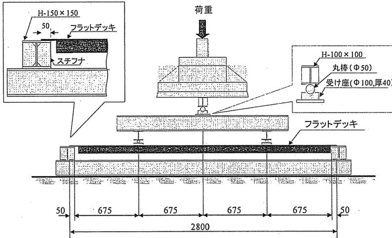
Fig.7 Bending tests.
