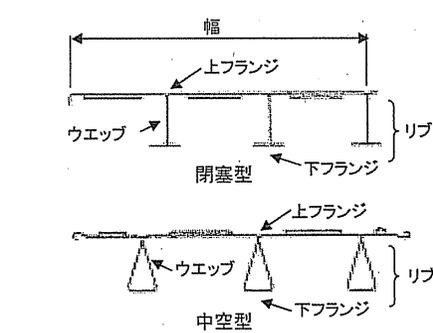
Fig.3 Section drawings of flat decks.
