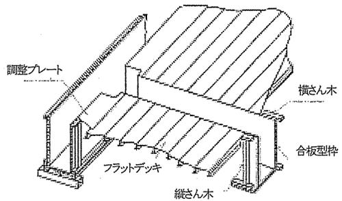
Fig. 1 Steel flat decks for reinforced concrete structure.
