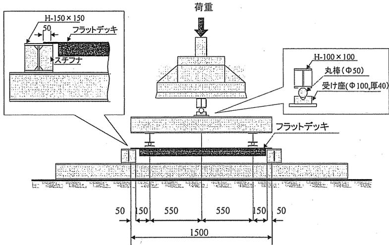
Fig.10 Strength test for end-closed of flat decks (bearing width 50mm).
