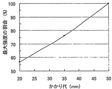
Fig. 18 Bearing width and maximum strength ratio.
